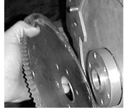
CAREFULLY ALIGN THE HUB SPACER/FLEX PLATE AND THE CRANKSHAFT BOLT HOLES WHILE PLACING THE HUB SPACER ONTO THE CRANKSHAFT. THE HUB SPACER SHOULD BE A CLOSE FIT TO THE CRANKSHAFT. INSTALL THE CRANKSHAFT BOLTS WITH THREAD LOCKING COMPOUND AND TORQUE TO THE PROPER VALUE.
