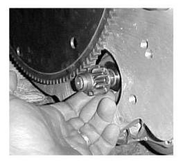
BEFORE INSTALLING THE TRANSMISSION, CHECK THAT THE TORQUE CONVERTER IS FULLY SEATED INTO THE FRONT PUMP OF THE TRANSMISSION. THE TORQUE CONVERTER MATING BOSSES SHOULD BE APPROXIMENTLY 1" FROM THE BELLHOUSING FACE.
