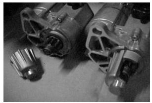
BECAUSE OF CLEARANCE, FOR YOUR APPLICATION YOU MUST MODIFY THE STARTER. THE "NOSE" OF THE STARTER MUST BE REMOVED. THIS REQUIRES THE USE OF A LATHE, BANDSAW, OR HACK SAW. MOST ANY MACHINE SHOP CAN PERFORM THIS OPERATION SAFELY AT A REASONABLE COST. WILCAP ALSO HAS THE MODIFIED STARTER AVAILABLE.
